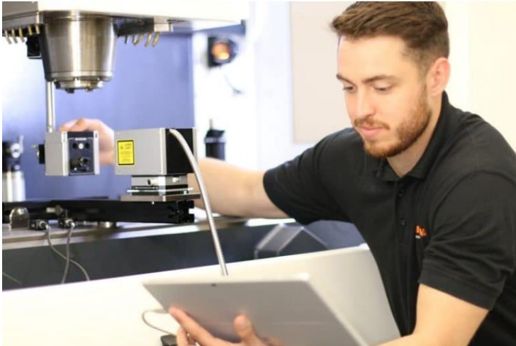
Calibration devices, such as this Renishaw XM-60 multi-axis calibrator, have become more powerful, yet easier to use. (Provided by Renishaw)
