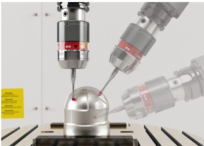
Okuma's Five-Axis Auto Tuning System uses a touch probe and a datum sphere to measure and auto-compensate for 11 types of geometric errors in about 10 minutes, or a fuller set of adjustments in 30 minutes. (Provided by Okuma)
